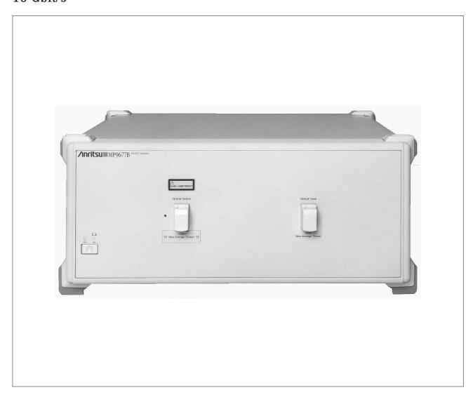
MP9677B is the 10 Gbit/s E/O and O/E converter for STM-64, OC-192 or FEC jitter evaluation and BER measurement. It has a jitter bandwidth of 80 MHz, and can measure jitter tolerance, jitter transfer, and output jitter at 10 Gbit/s optical interface when used with MP1777A. It can be also used with MP1570A.
